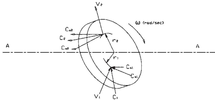
**Figure 1.17** Velocity components for a generalized rotor.
