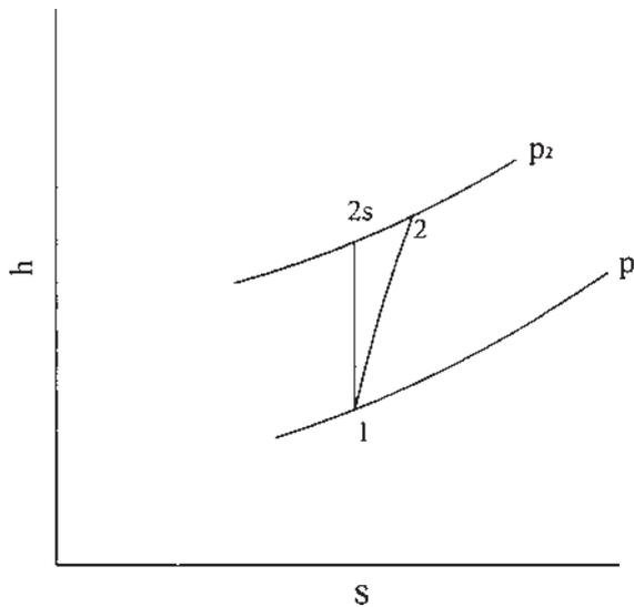
**Figure 1.16** Mollier diagram for the diffusion process.
