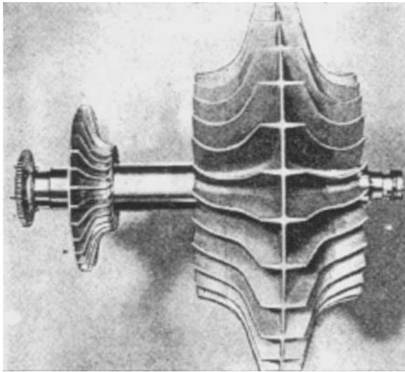
**Figure 1.3** Centrifugal compressor rotor (the large double-sided impellar on the right is the main compressor and the small single-sided impellar is an auxiliary for cooling purposes). (Courtesy of Rolls-Royce, Ltd.)
